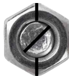
(Bolt is loose)
